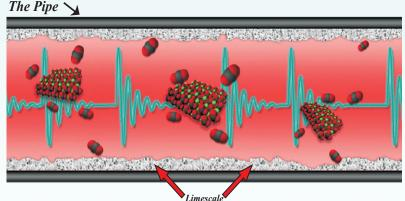
Hydrokon treats fluids by inducing a electrostatic field of 7k to 12k DC volts, yet harmless fields throughout plumbing pipe lines/systems made of any material, including PVC. When the Hydrokon signal is present, dissolved minerals combine to form loosely held clusters.
